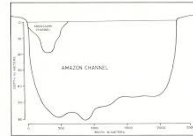
Fig. 1. Cross-section of the bed of the Lower Amazon near Óbidos (its narrowest place) compared with that of the Mississippi at Vicksburg. After Davis 1864.
